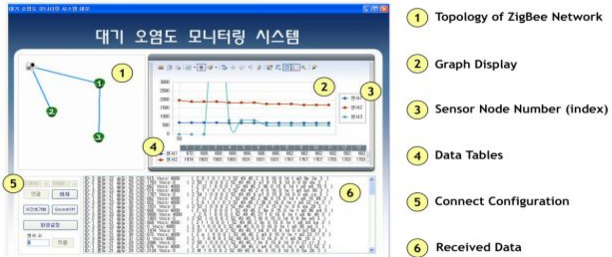
Figure 6. Screen shot of an IAQ monitoring system
